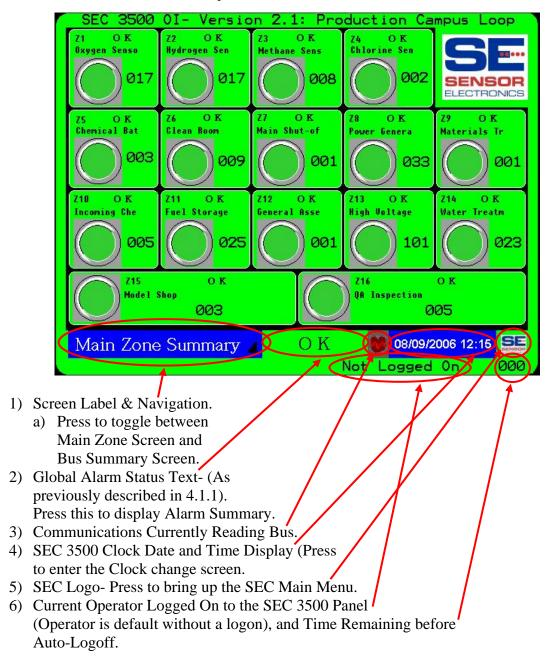
Important Note: It is important to realize that the bottom status bar region remains constant for all of the main operations screens, along with the global status bars and status text. The only difference will be the screen name in the lower left corner. If the screen name is followed by a navigation the above screen), then it allows rapid navigation between it and the Bus Summary screen.
