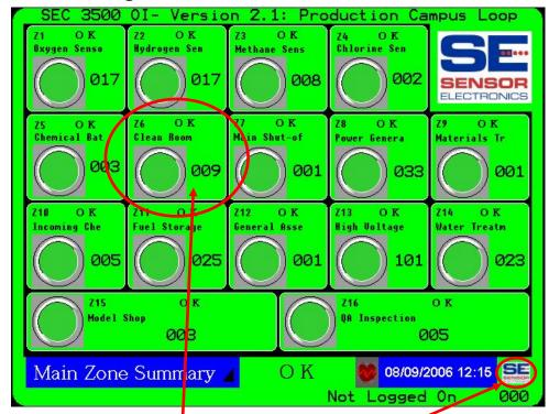
Simply press on the desired zone box, or bring up the Main Menu and select "Select Screen", then "Zone Details", then the desired zone number/name then press "Select".
